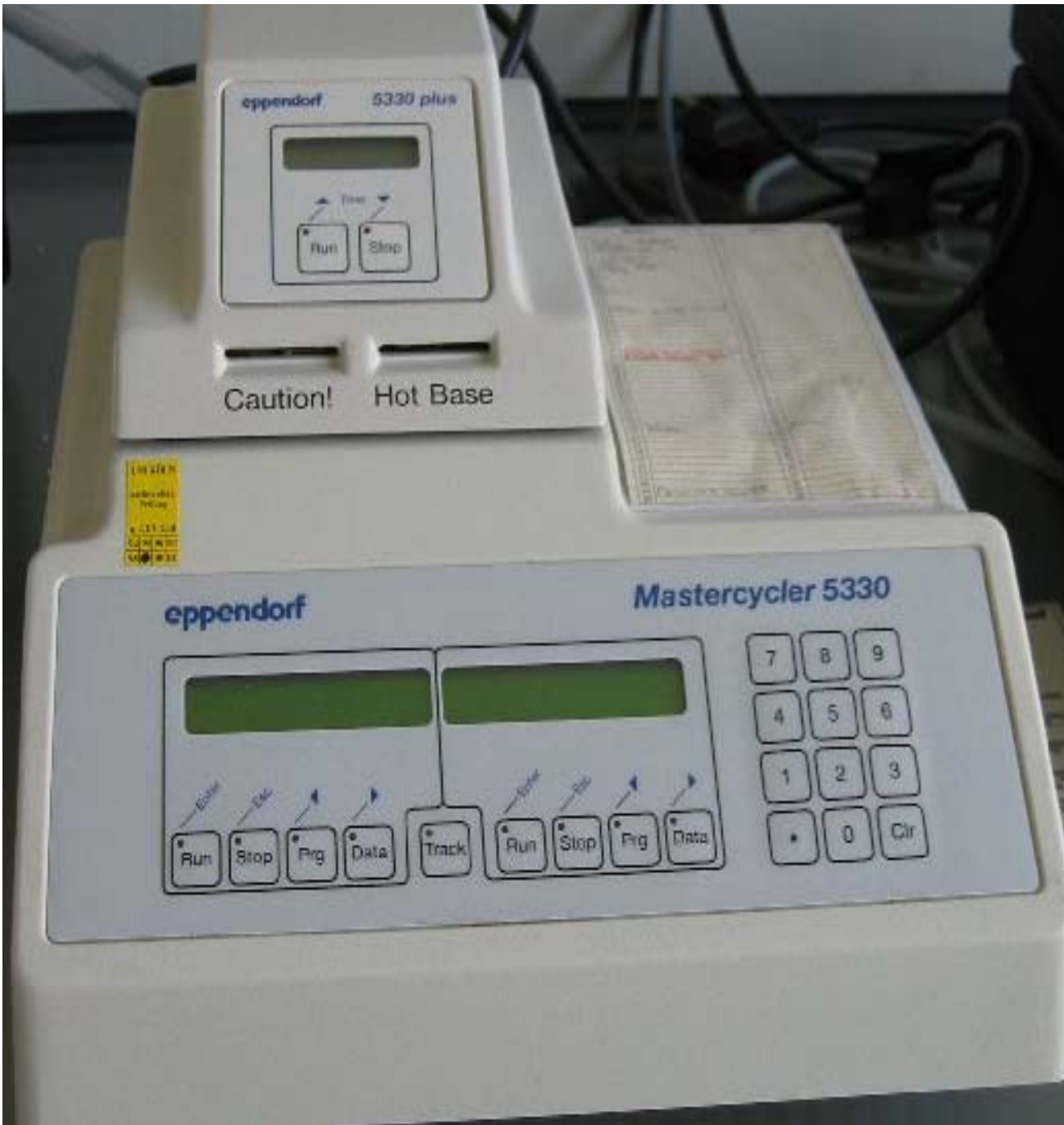
FIGURE I : Thermal Cycler (PCR Machine) picture is an example of the machine that has a heating block and an operating system. This allows programming the heat block and vary temperature, following a cyclic program
