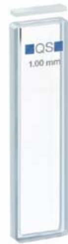
Figure 5 Quartz SUPRASIL Fused Silica 1mm Cell
