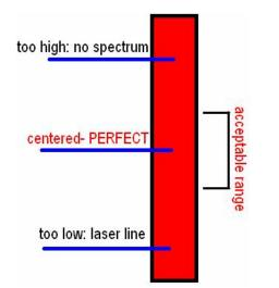
The laser must be a single dot, the diameter measurable in only micrometers, in the center of the slit. When the laser hits the slit, it goes into the spectrograph, where the changes in vibrational energies are measured.
