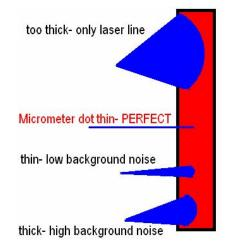
Therefore, focusing the laser into the slit perfectly is crucial to the spectrum. If the laser is diffuse, then there will either be a very high background, which blocks any possible peaks. If it is too high or too low, there may not even be a spectrum.
